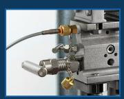
High Pressure Hoses & Quick-test Connections
