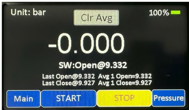
1st switch status: open at 9.332 bar
