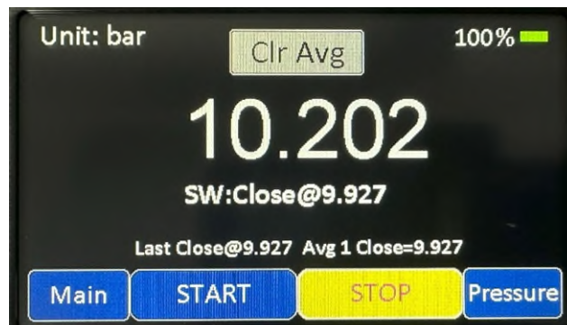
1st switch satus: close at 9.927 bar
